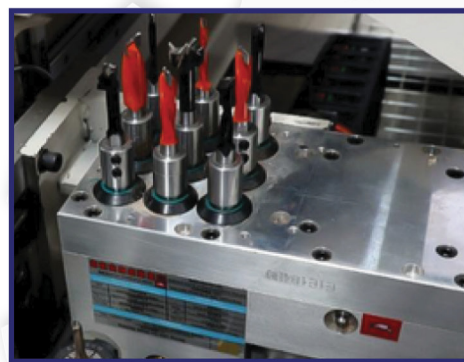
Lower drill unit: 9 vertical drills+One 3.5kW spindle
