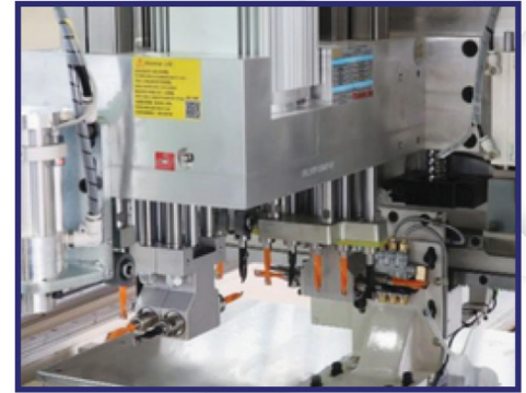
Upper drill unit: 12 vertical drills+8 horizontal drills+ One 3.5kW spindle
