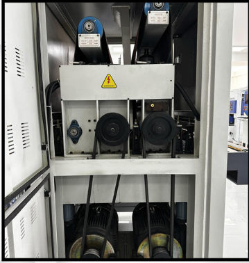
The first sand frame-steel roller
