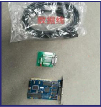
NC Studio control system
