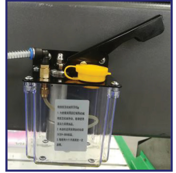
Manual oil lubrication system
