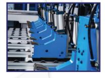
In the cutting area, tables with an air cushion are also installed, which greatly facilitates the work with small parts and protects them from damage.
