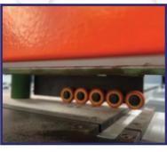
Side stops precisely position narrow strips along the side ruler when cutting them into finished parts (optional).
