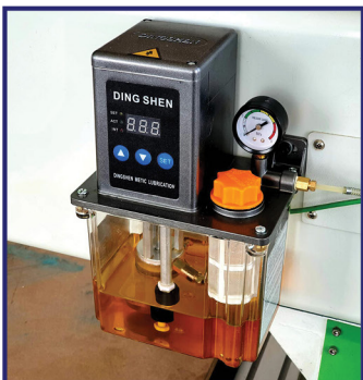
Automatic oil lubricating system
