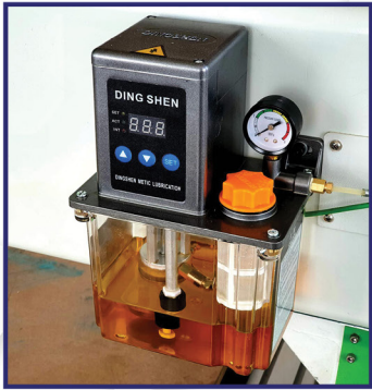
Automatic oil lubrication system prolong service life
