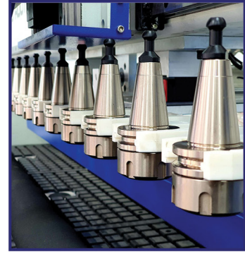
12 tools for auto change with linear-type
