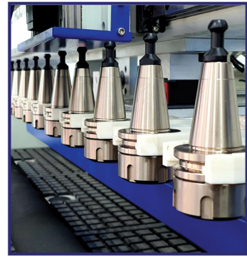
12 tools for auto change with linear-type
