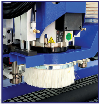
9kW air cooling spindle
