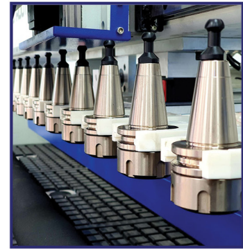
12 tools for auto change with linear-type
