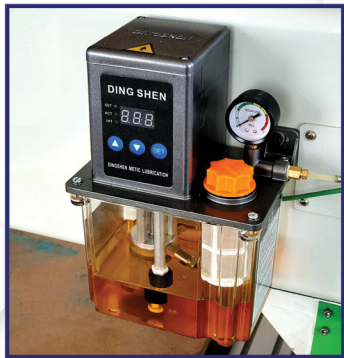
Automatic oil lubrication system prolong service life
