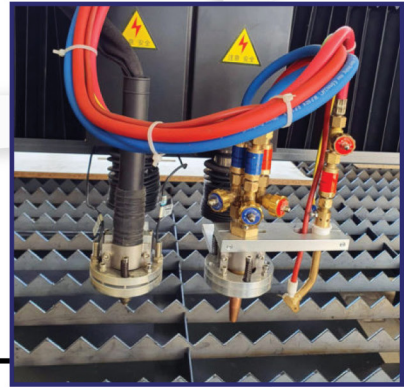
Optional flame cutting for thicker plates
