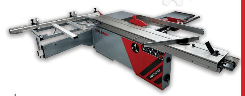
The HOLZMANN panel saw HM305V32TOP with 3.2m sliding table, scoring unit (height and side adjustable), main saw blade with height and angle adjustment, table extension, outrigger table - a perfect saw for processing your panels in your joinery workshop.
