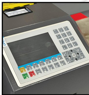
Industrial RUIDA controller
