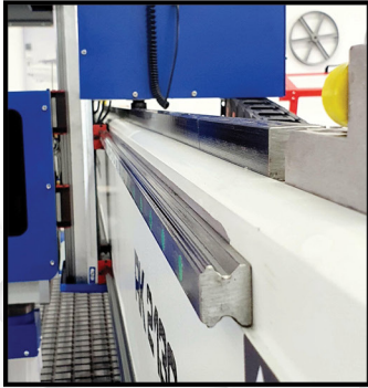
HG20 Taiwan HIWIN square rails, tilted teeth rack
